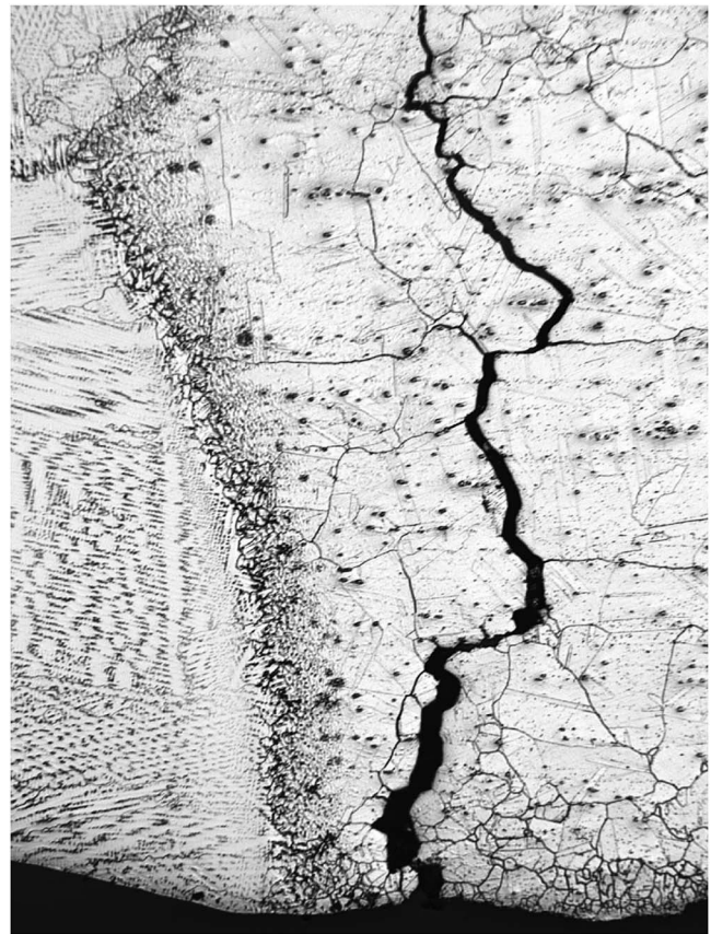
Fig. 4 Strain-age cracking of a simulated repair weld in R-41 alloy
